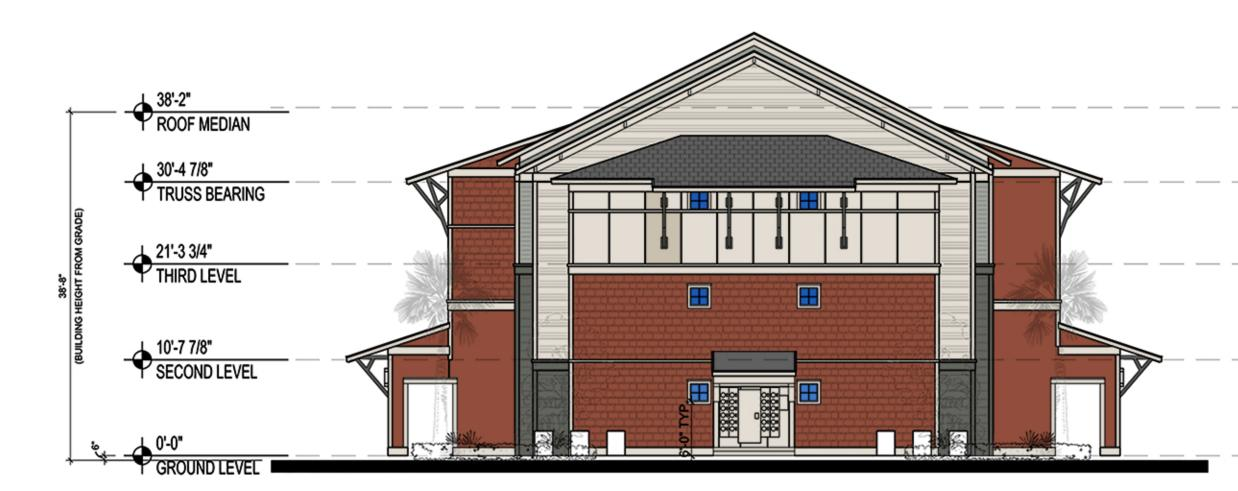
**BUILDING #3 (TYPE 3) - EAST ELEVATION SCALE:** 3/32" = 1'-0"
