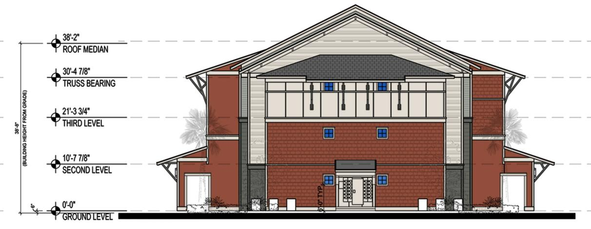
**BUILDING #3 (TYPE 3) - WEST ELEVATION SCALE:** 3/32'' = 1'-0''
