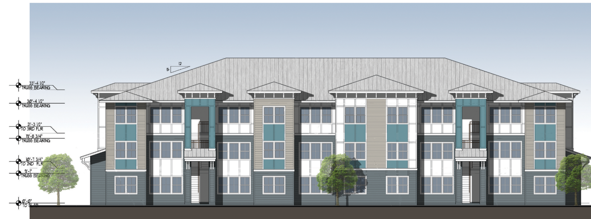
1 FRONT ELEVATION OF BUILDING NO'S. 1, 4 & 5 SCALE: 1" = 1/8"=1'-0"
