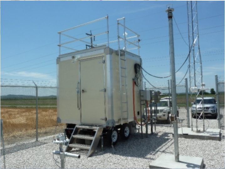
Traditional EPA RM Monitoring Station (Mobile)
